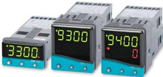
The West CAL Series Controllers provide essential temperature control functions including heat/cool operation and a simple ramp/dwell program. Integrated auto-tune optimizes PID settings and a unique dAC function minimizes overshoot. Each model accepts thermocouple (9 types), Pt100 RTD and mV inputs. Two relay outputs and Modbus communication (RS-232 or RS-485) are optional. The 1/32 or 1/16 DIN case has an IP66 front and UL/cUL certification.
