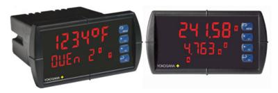
New models in the YPP Series expand measurement ranges to 300V and 5A AC/DC. These dual input meters are ideal for reading direct inputs or signals from shunts and current transformers. A math channel calculates apparent power. The YPP6400 can display any two parameters (V, A, VA) or alternate between the parameters.
