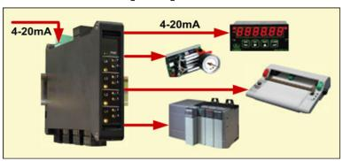
The Laurel QLS Quad Loop Splitter sources four separate 4-20mA outputs from a single input. Outputs can have the same ground or grounds differing by up to ±10V. Benefits of a loop splitter include:
