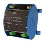
The **NK Technologies** VTU family of voltage transducers provide high accuracy and safety in a panel or DIN-rail mounted housing. One sensor can measure DC or AC circuit voltages to 1200V. The VTU modules are externally powered from 24V AC/DC and generate an isolated process output of 0-5V, 0-10V or 4-20mA. They are UL listed and CE compliant.
