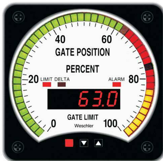
Bar changes color when gate position exceeds limit. UP button toggles digital display between position, limit & delta. Example of a custom dial shown here.
